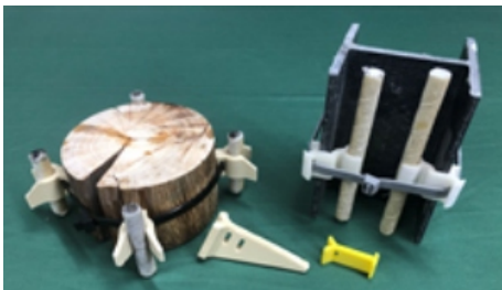
Fig. 3. Sample spacers and skirt pin.
