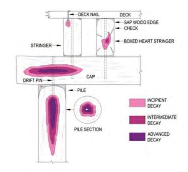
Shows the level of decay that occurs in timber due to the use of vertical fasteners. Vertical fasteners increase the rate of decay in timber as they allow moisture to travel down the fastener into the heartwood of the cap, stringers, corbels and piles, therefore increasing the moisture content in the middle of these elements.
