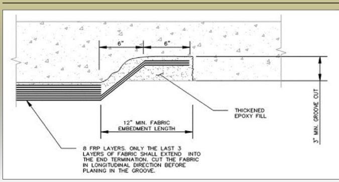
Figure 5. Termination detail for the 8-layer StifPipe® used for the I-35 tunnel repair.
