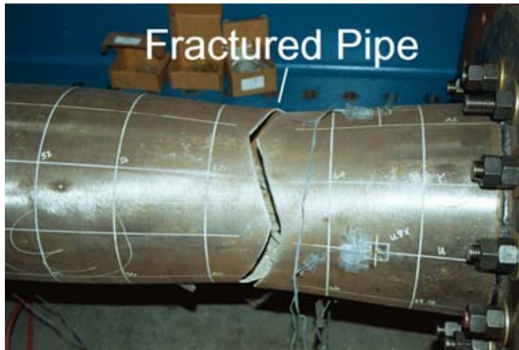
Figure 9. Specimen 12.3. Fractured Pipe.
