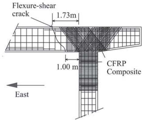
Figure 18 - Flexure-shear crack at cap beam of West column at 6% drift ratio – 2000 tests.
