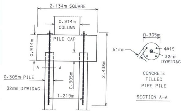
Figure 6 - Detail of pile-to-pile cap connection – 1998 tests.
