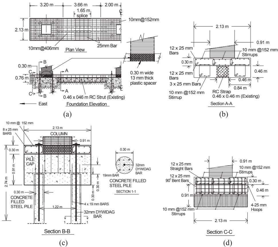
Figure 13 - Grade beam for 2000 tests: (a) plan and longitudinal section, (b) grade beam section A-A, (c) grade beam-to-pile section B-B, (d) end beam section C-C.
