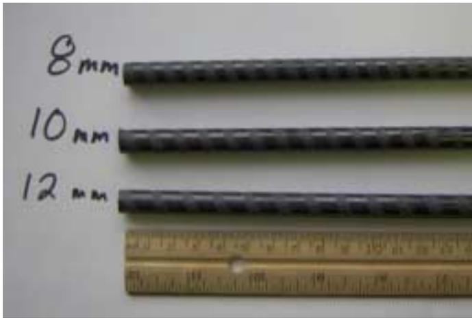
**Figure 1.** CFRP reinforcement with spiral indentation pitch lengths of 8 mm, 10mm and 12 mm.
