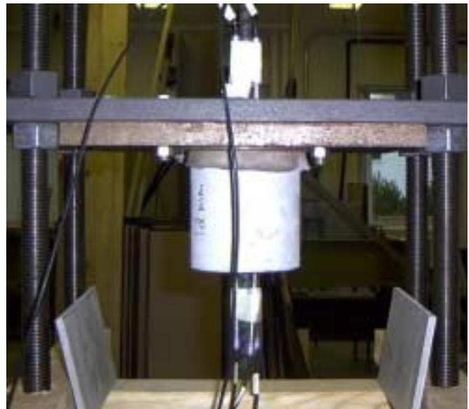
**Figure 2.** Bond Strength Test Set-up.
