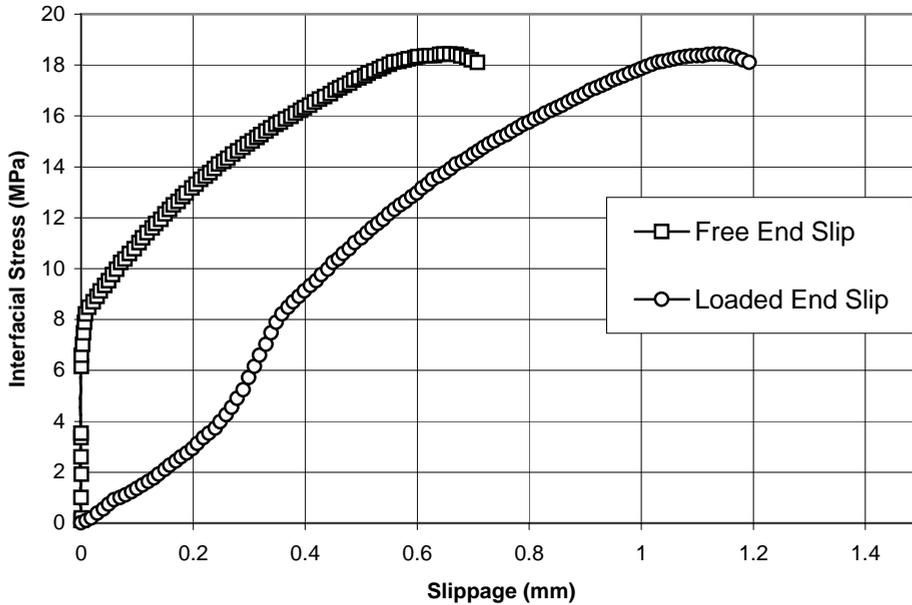
**Figure 4.** Typical CFRP Interfacial stress vs. slippage (8mm pitch length).
