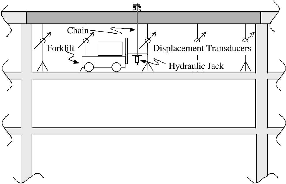
Figure 2.5: Pull-down test configuration with a mobile reaction
