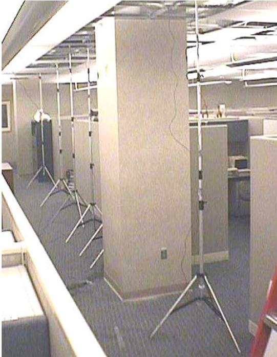
**Figure B.5: LVDTs mounted on aluminum tripods**
