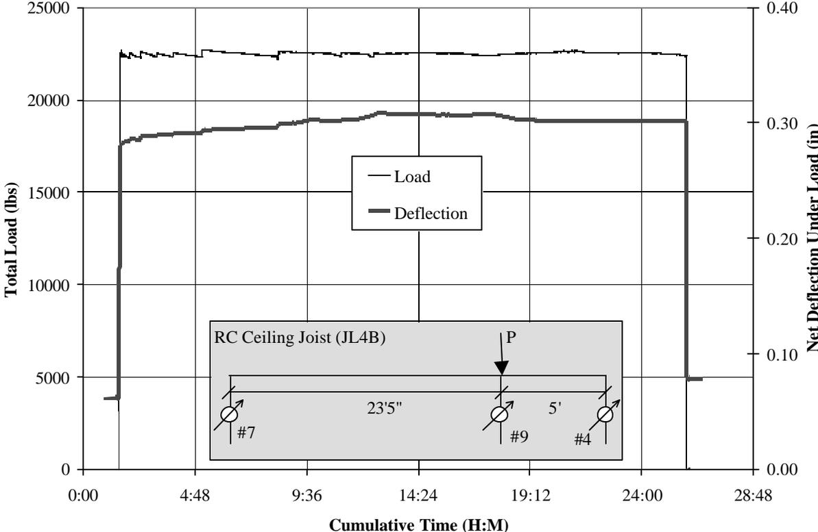
**Figure A.24: Time history of 24-hour load test for JL4B**
