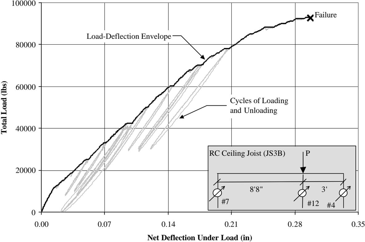
**Figure A.13: Load versus deflection curve for JS3B**
