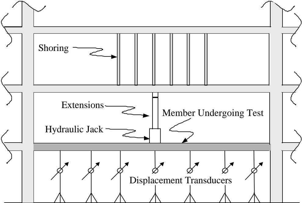
Figure 2.1: Push-down test configuration
