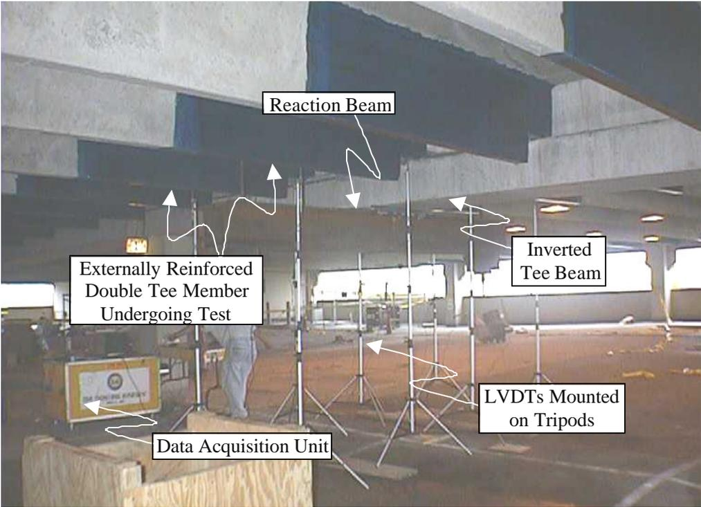
**Figure B.16: Closed loop method from below the test members**
