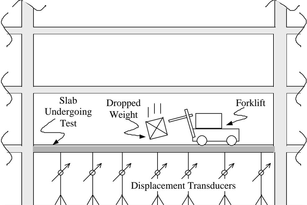
Figure 2.12: Load test configuration for a dropped weight
