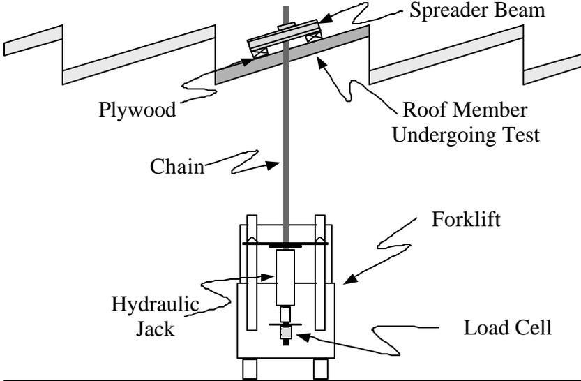
Figure 2.6: Detail of pull-down test method with a mobile reaction
