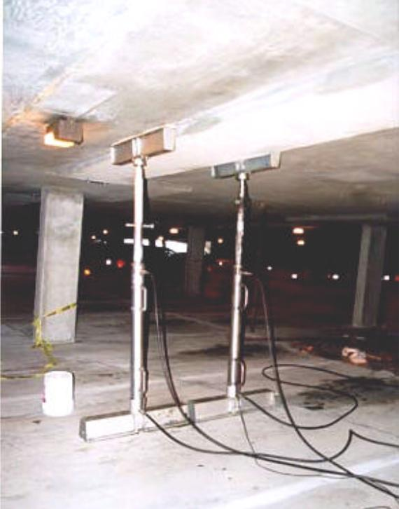
**Figure B.1: Load applied by hydraulic jacks**
