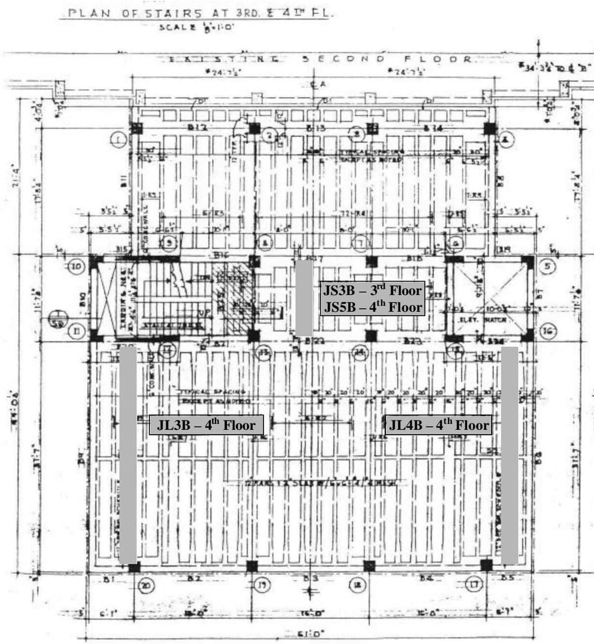
Figure A.7: Plan view shows locations of tested members
