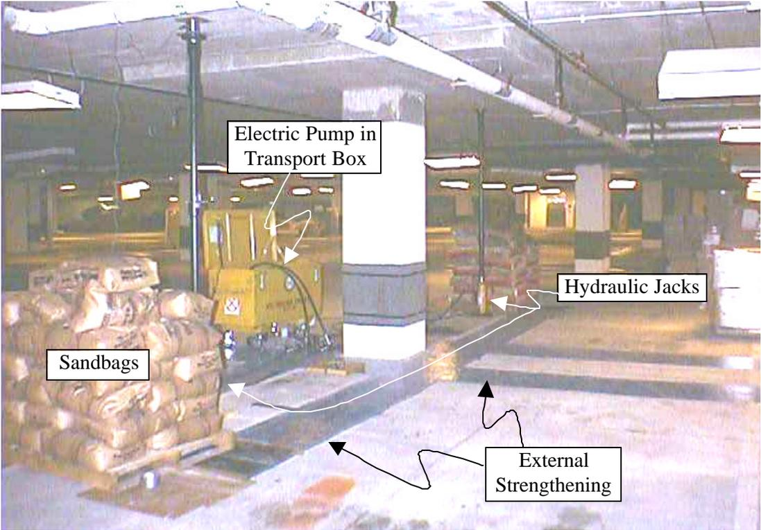
**Figure B.3: Load applied using hydraulic jacks and sandbags**
