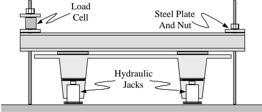
Figure A.2: End view of setup for testing of PC double tee
