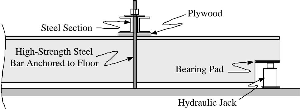
Figure A.1: Side view of setup for testing of PC double tee
