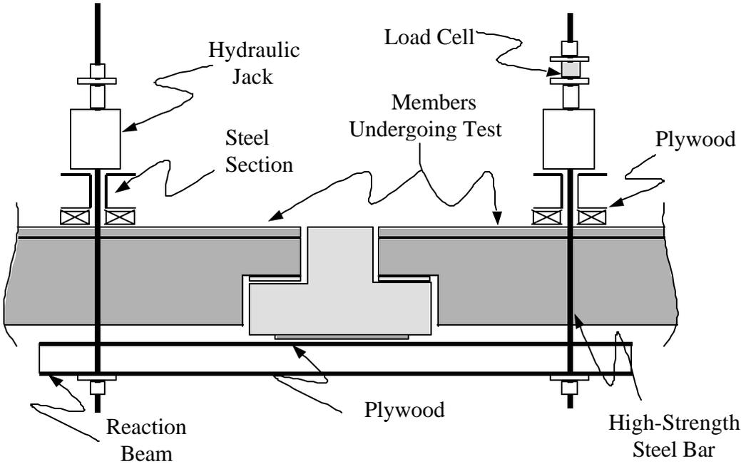
Figure 2.8: Detail of loading devices for the closed loop method
