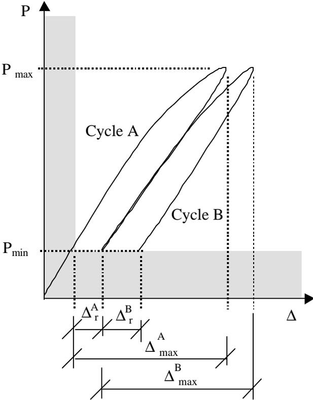
Figure 3.2: Sample load versus deflection curve for two cycles
