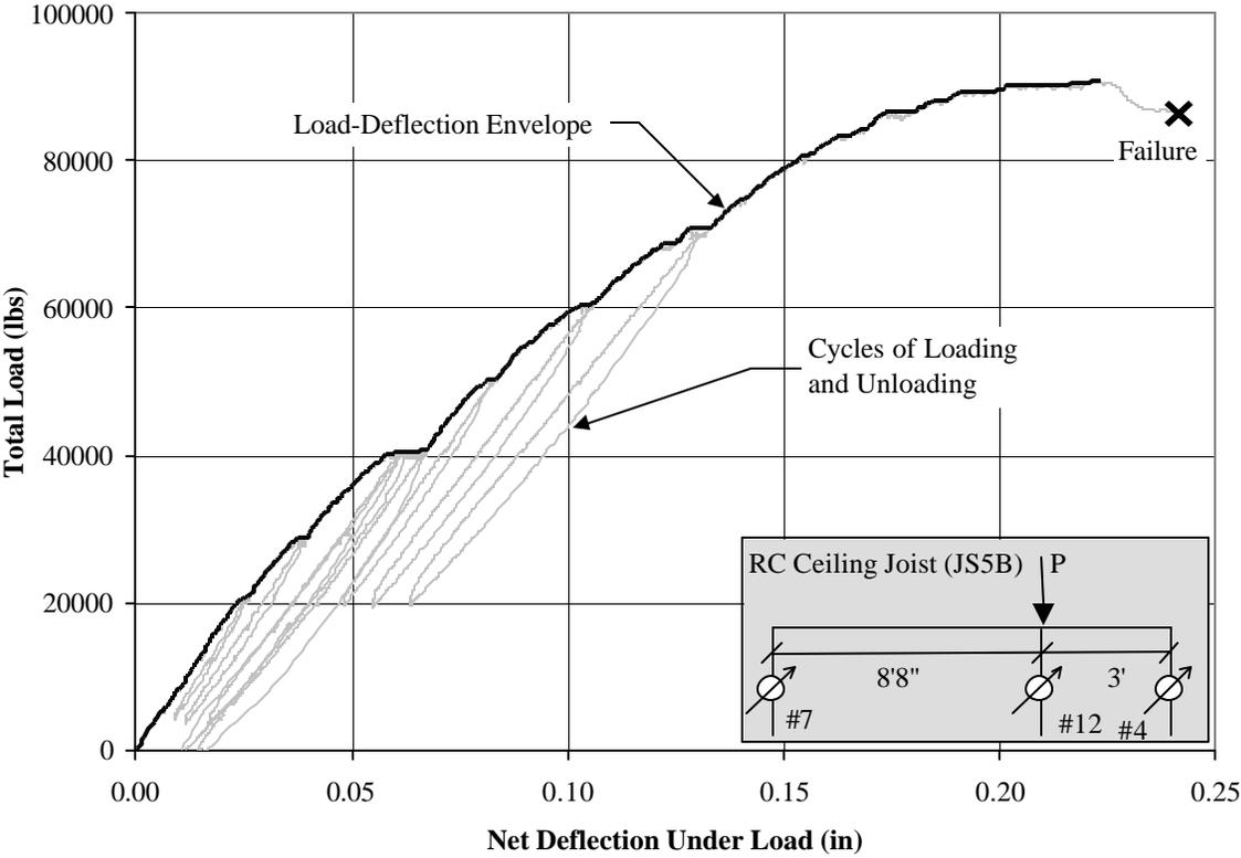
**Figure A.19: Load versus deflection curve for JS5B**
