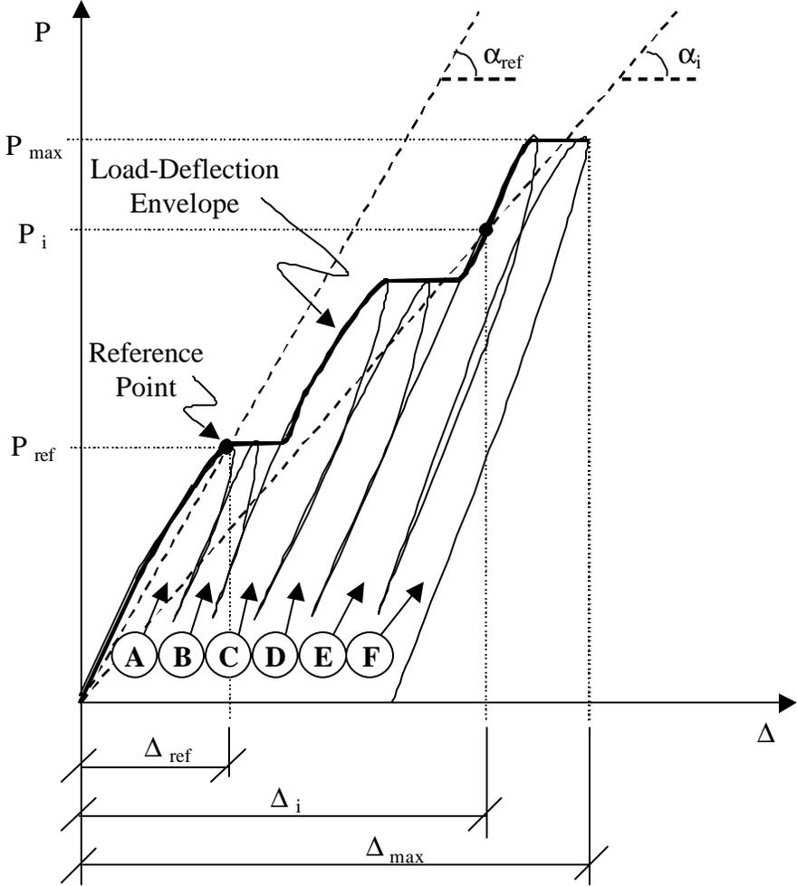
Figure 3.3: Sample load versus deflection curve for six cycles
