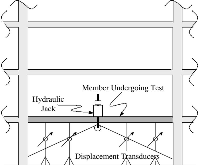
Figure 2.3: Pull-down test configuration with a fixed reaction
