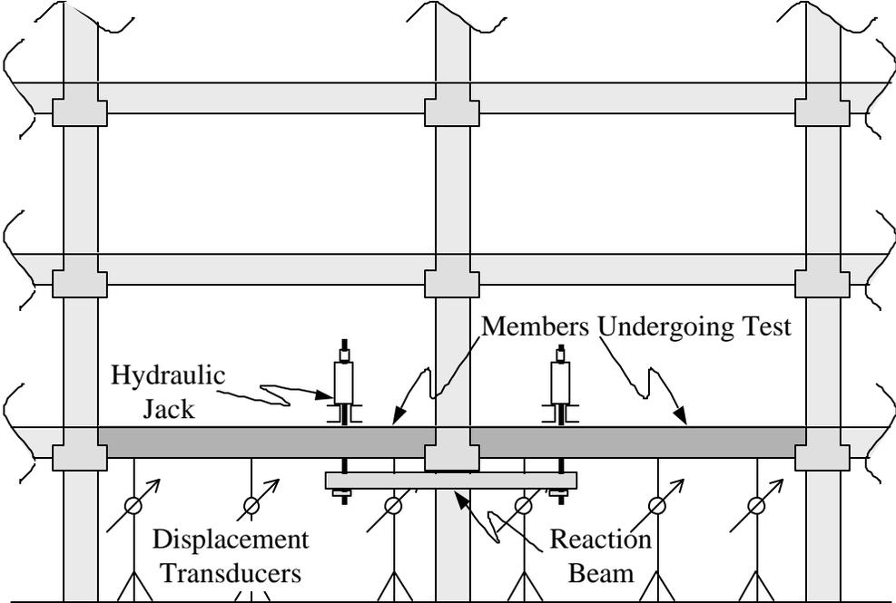
Figure 2.7: Closed loop test configuration
