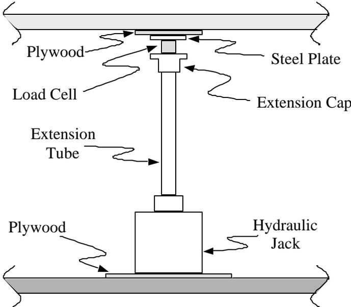
Figure 2.2: Detail of push-down test method
