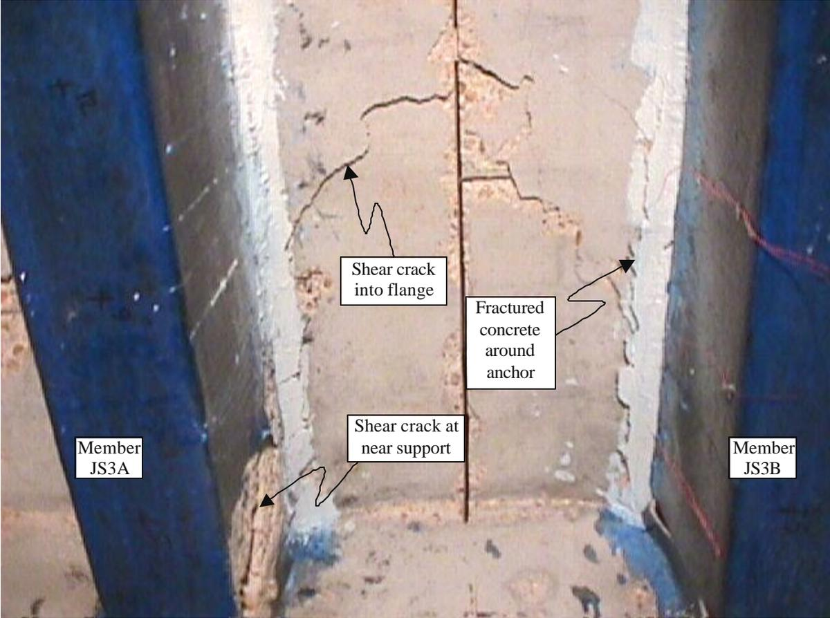
Figure A.16: Failure of members JS3A and JS3B
