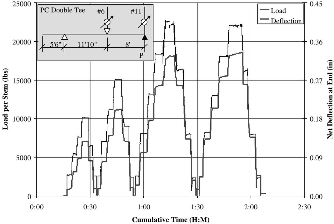
**Figure A.3: Time history of rapid load test for PC double tee**
