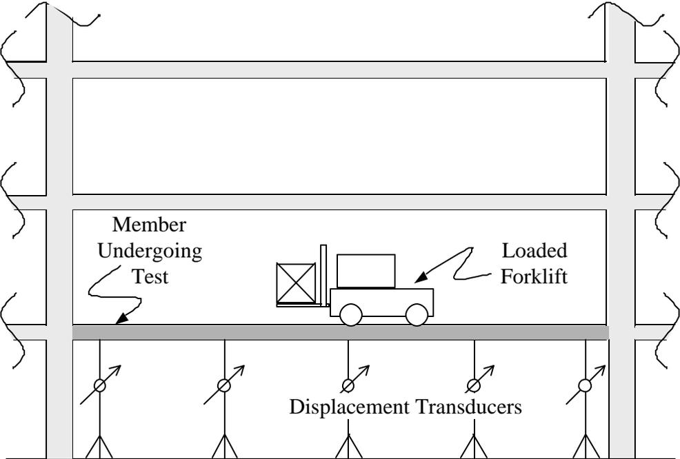
Figure 2.10: Vehicle loaded test configuration
