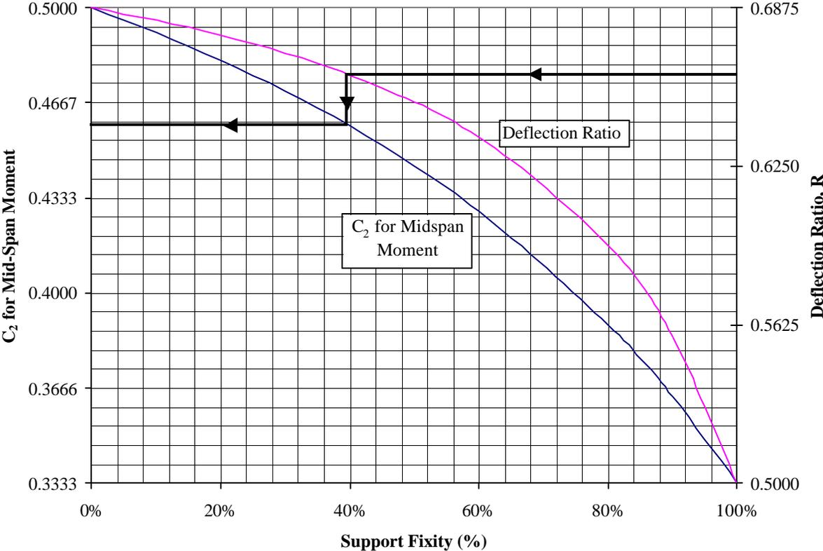
Figure 3.4: Variation of  $C_2$  and  $R$  for a symmetrically bound member loaded at mid-span
