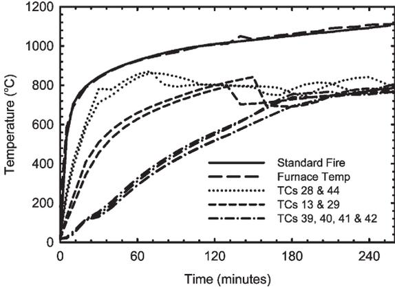
Fig. 4—Temperatures recorded at various locations in column SQ1 as a function of fire exposure time
