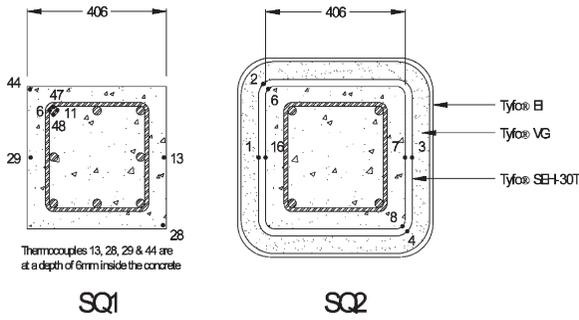
Fig. 2—Thermocouple locations in Columns SQ1 and SQ2 at mid-height
