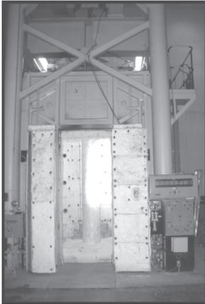
Fig. 3—The NRC Column Furnace with a columns installed prior to testing
