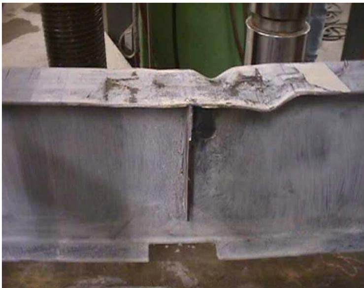
**Figure 4-12 Failure Mode of Test Unit 2**
