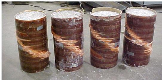
**Figure 5-12 Typical Failed Specimens**
