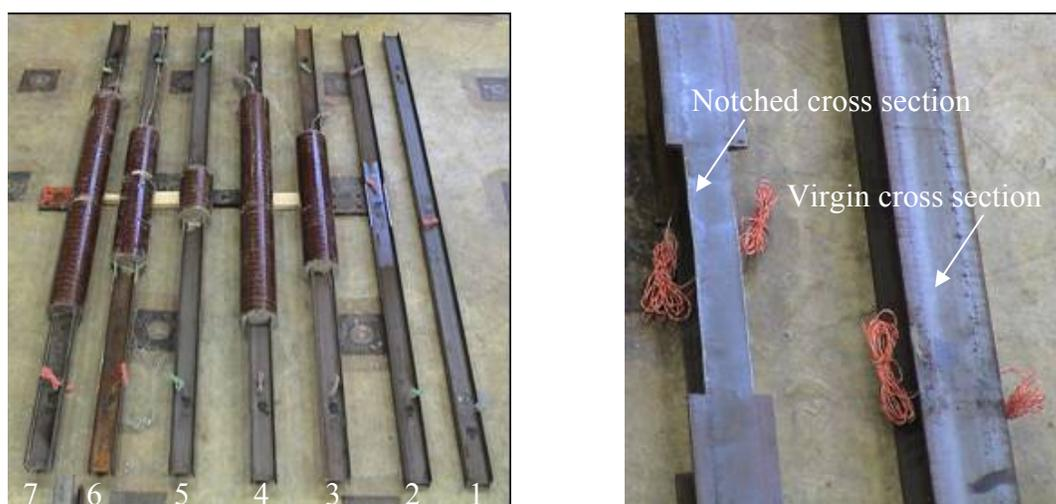
**Figure 5-25 Test Specimens**
