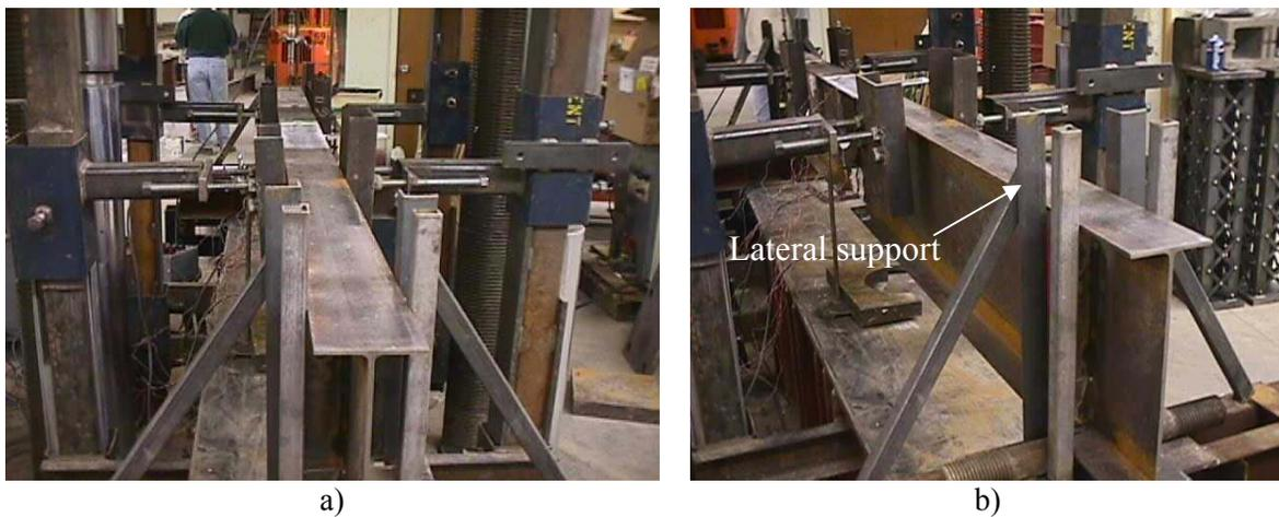
**Figure 4-7 View of Lateral Support Setup**
