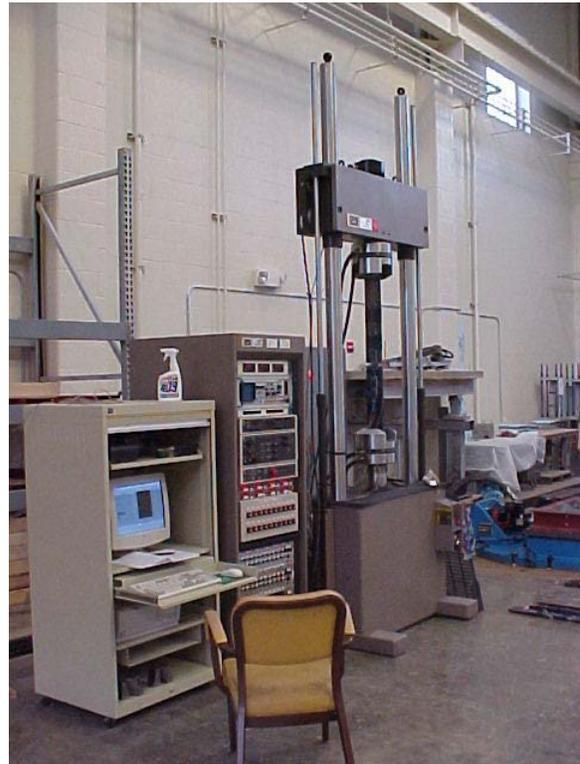
**Figure 3-5 MTS 880 and Data Acquisition**
