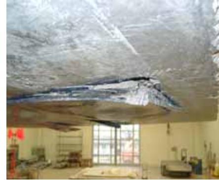
f) Failure of anchoring: pull off of the concrete cover
