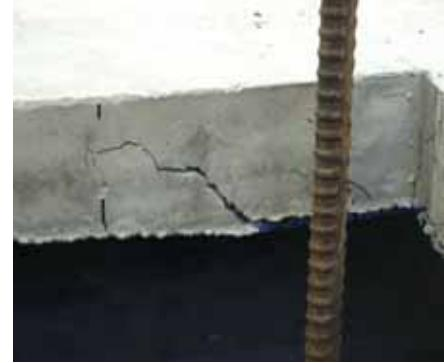
d) Shear crack in the opening
