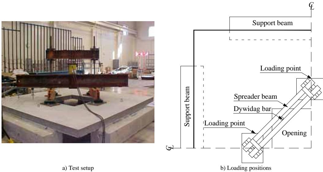
Figure 3 - Test setup
