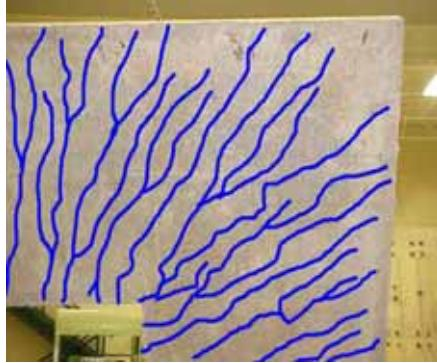
c) Typical crack pattern on bottom of the slab
