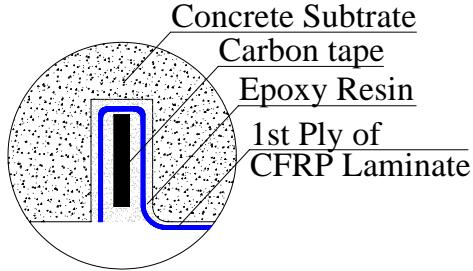
Figure 2 - CFRP Laminates application by manual wet lay-up on tension side of specimen SQ3
