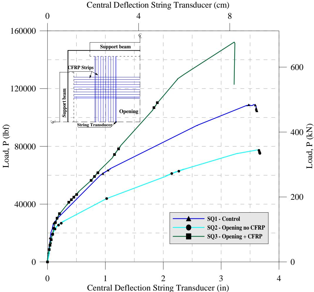
Figure 5 - Load vs Deflection curves
