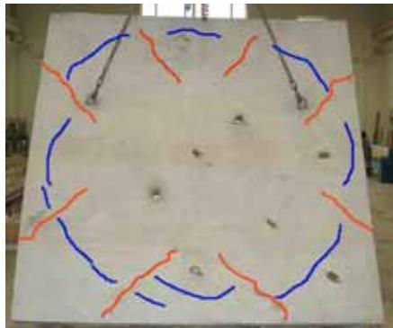
a) Top cracks in solid slab
