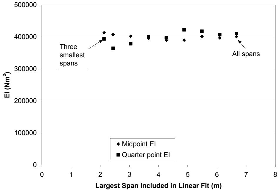
Figure 8: Sensitivity of EI on largest span included in linear fit (connected panels)
