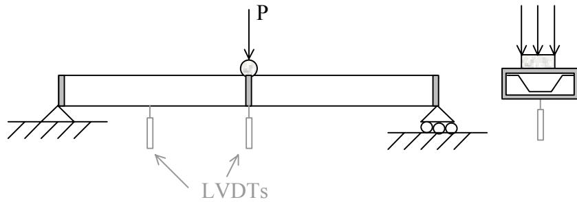
(a) Three-point bending set-up for single panel tests
