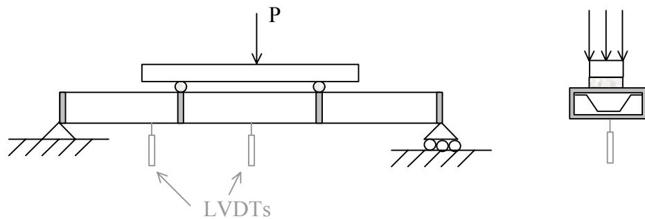
(b) Four-point bending set-up for both single and double panel tests
