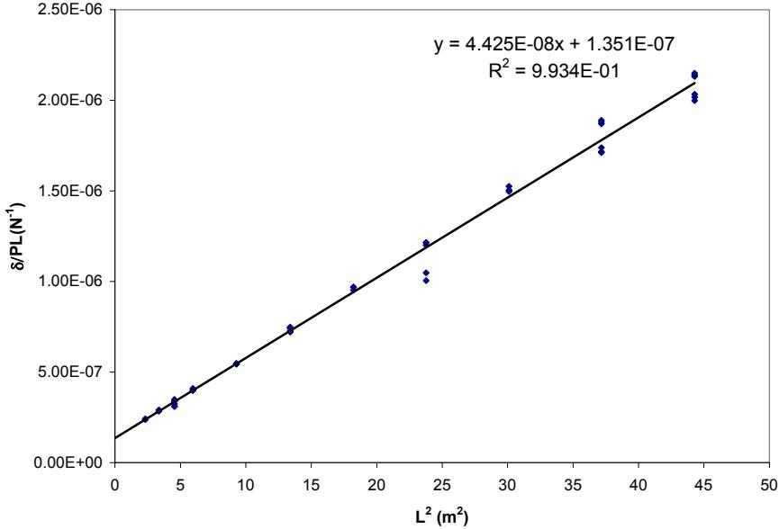
Fig. 6: Straight line used to determine the flexural rigidity from four-point bending based on the midpoint deflection (connected double panels)
