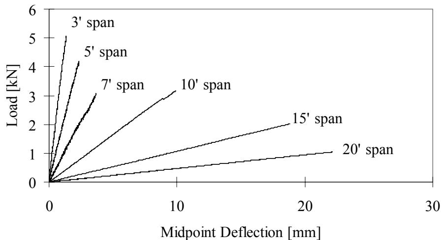
Figure 3: Typical load-deflection curves at the midpoint for four-point bending linear tests (single panel,  $1' = 0.3048\text{m}$ )
