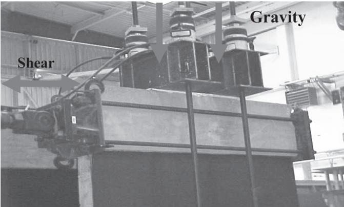
Figure 2 – Gravity and Cyclic Shear Loading on Typical Wall.
