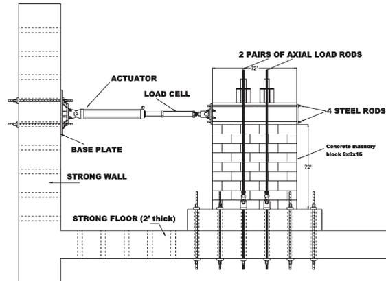
Figure 1 — Test Set-Up.
