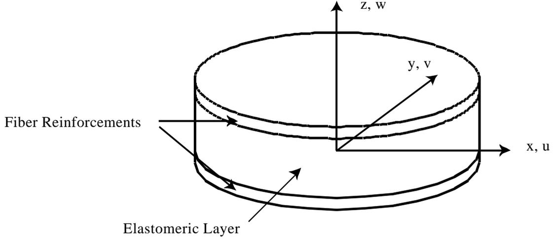
**Figure 1.** Elastomeric layer with fiber reinforcements
