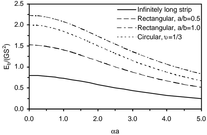
**Figure 3.** Variation of effective bending modulus with  $\alpha a$
