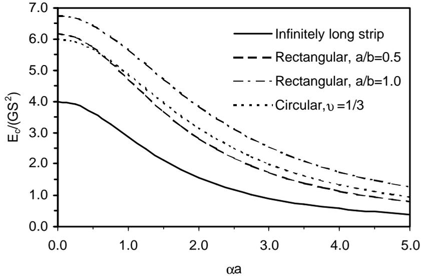
**Figure 2.** Variation of effective compressive modulus with  $\alpha a$
