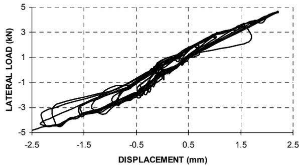
**Figure 3.** Bending Baseline Specimen Results
