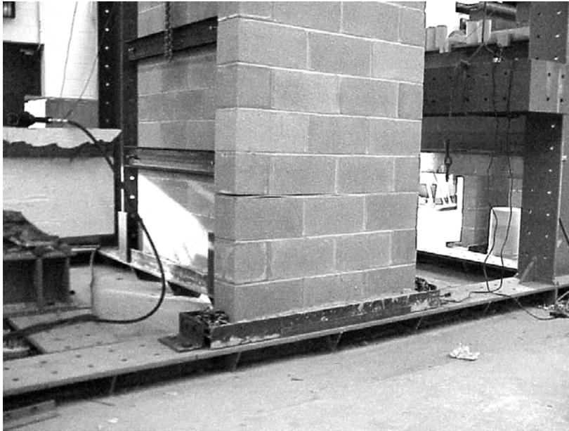
**Figure 1.** In-plane Baseline Shear Specimen at Failure
