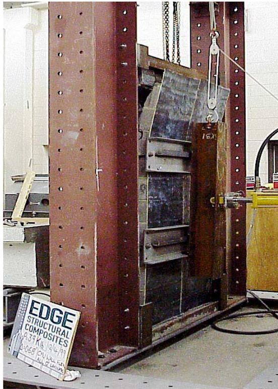
**Figure 7.** Retrofitted Bending Specimen at Failure
