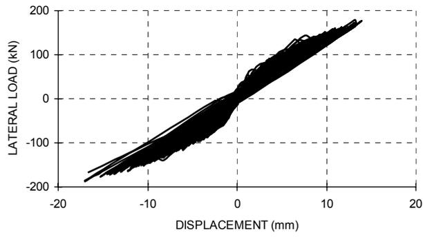
**Figure 6.** Retrofitted Bending Specimen Results
