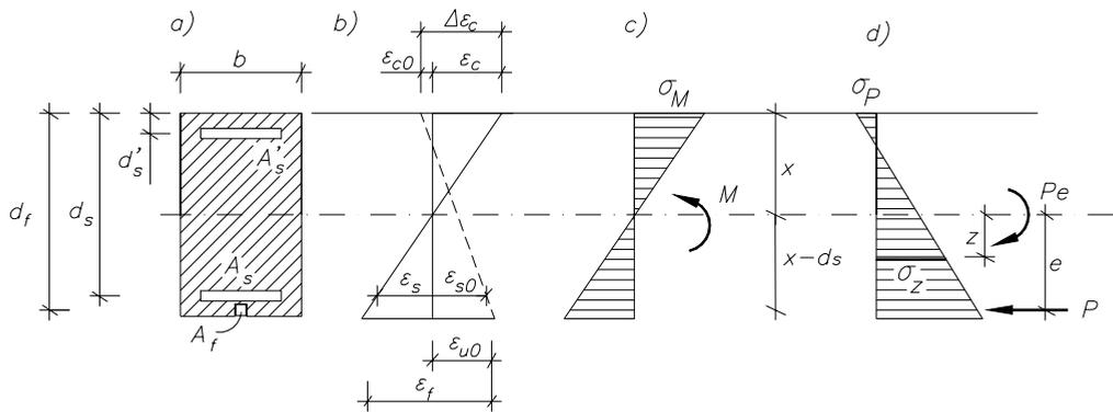
**Figure 2.** Stresses and strains acting on a pre-stressed rectangular cross-section
