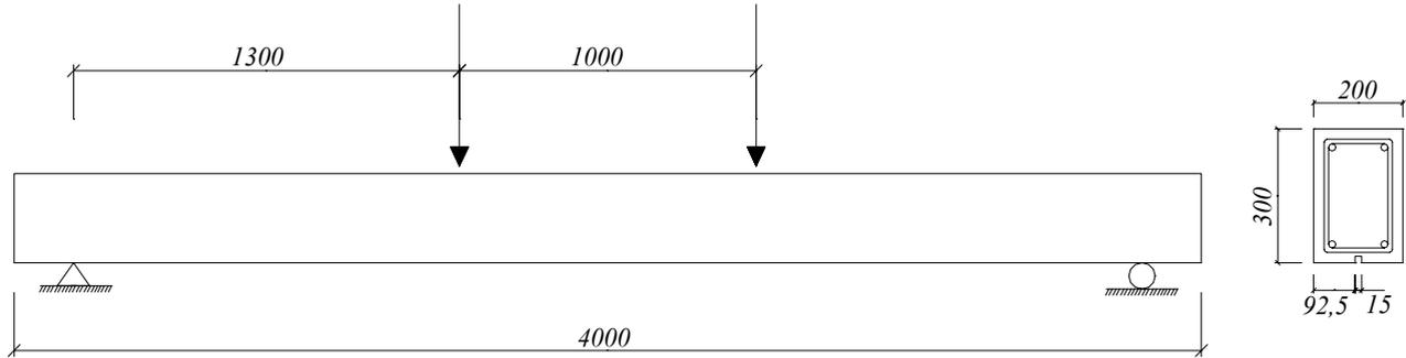
**Figure 4.** Beam test setup
