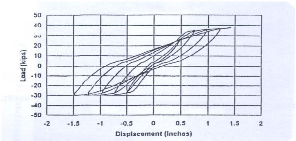
**Figure-1** Load-Deflection plot for the control specimen SP-1
