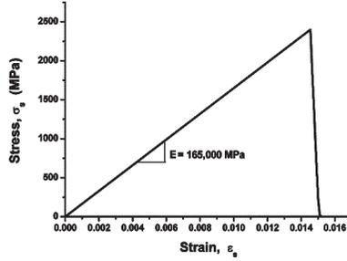
Figure 4 – Property of CFRP laminate
