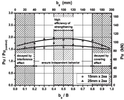
Figure 10 – Comparison of ultimate load by groove depth relative to spacing ratio
