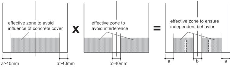
Figure 11 – Disposition to ensure independent behavior of the CFRP reinforcements
