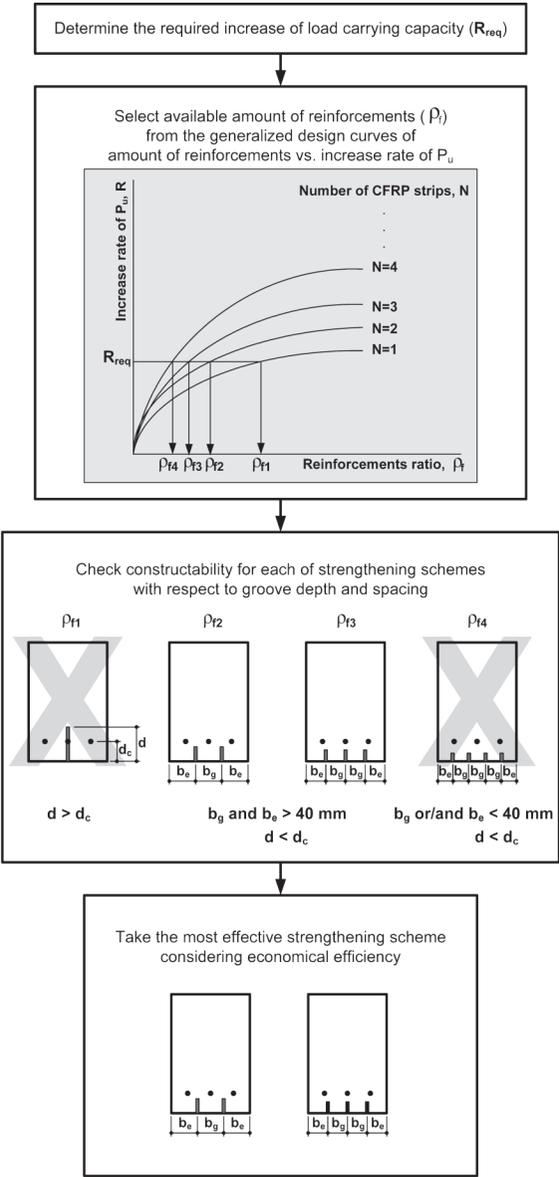
Figure 12 – Conceptual design flow of NSM reinforcement
