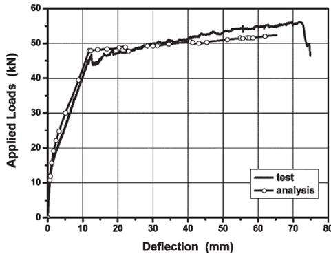
Figure 6 – Comparison of analytic and experimental results for CONTROL
