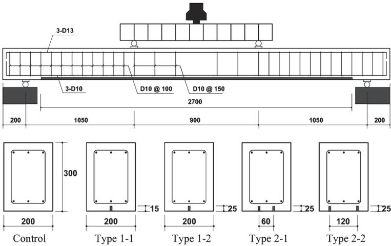
Figure 1 – Test set-up and specimen details
