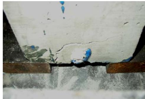
**Figure 11. Anchorage Failure Mode**
