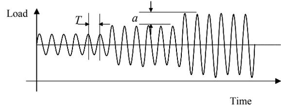
**Figure 9. Dynamic Bond Test Loading**
