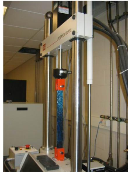
Figure 4. Test Setup for VE Specimens
