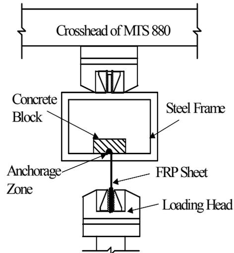
Figure 5. Anchorage Test Setup
