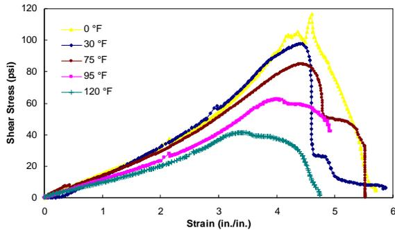
**Figure 8. Stress-strain Curves under Static Loading**
