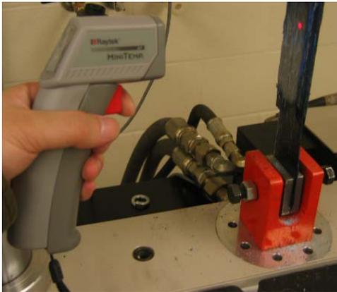
Figure 6. Infrared Thermometer
