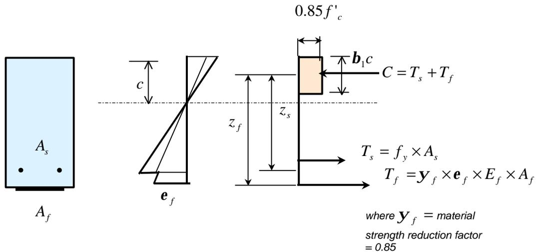
**Figure 6.3: Design Moment less than Balanced Failure Moment using ACI 440 Draft Guidelines and ACI 318**
