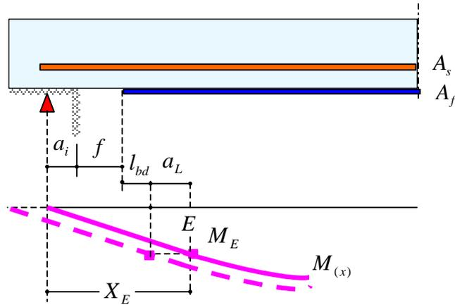
**Fig 6.6: End support conditions for bond development**
