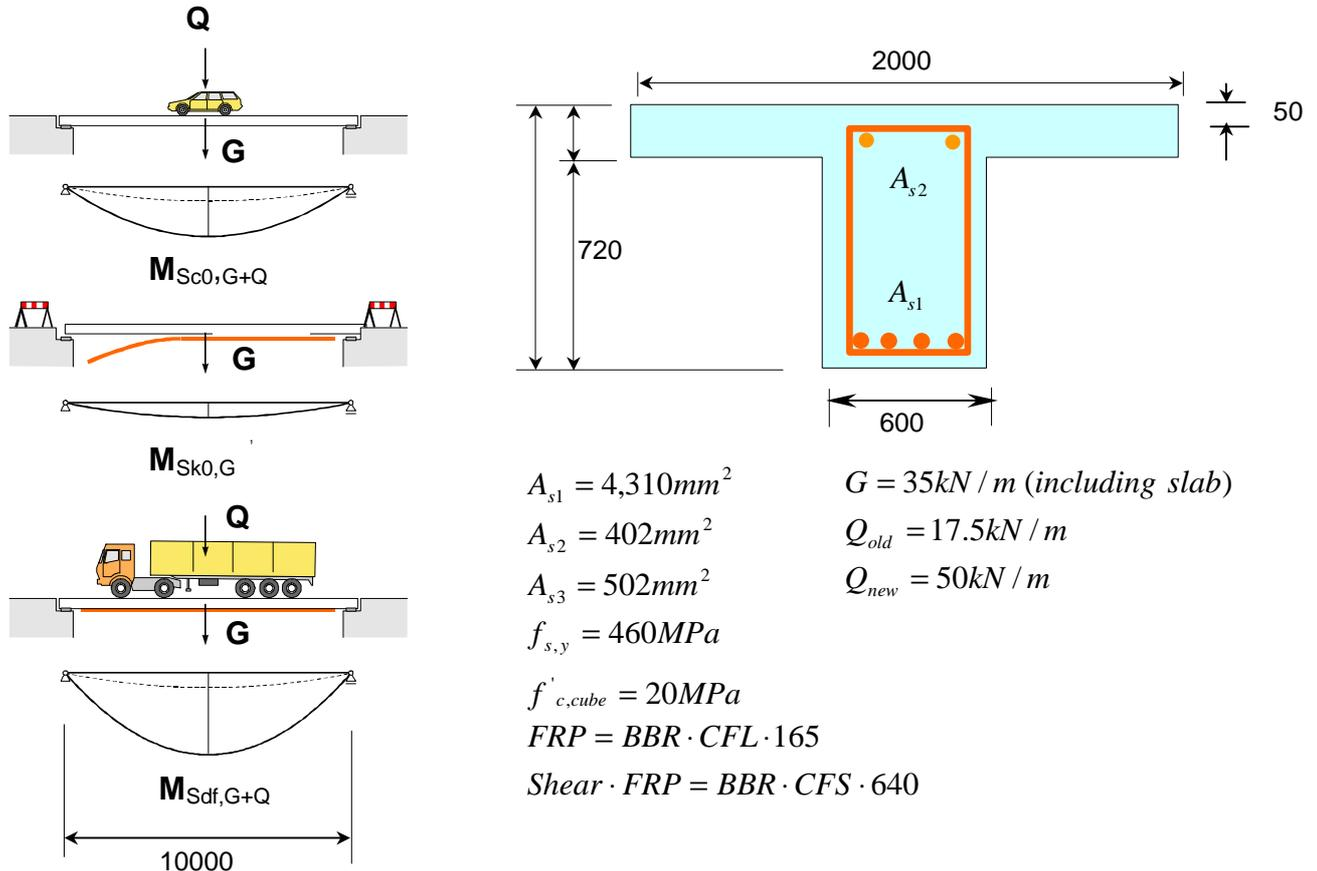
Find the required strengthening using BBR CFL 165 laminates for flexure and BBR CFS 640 sheet for shear.
