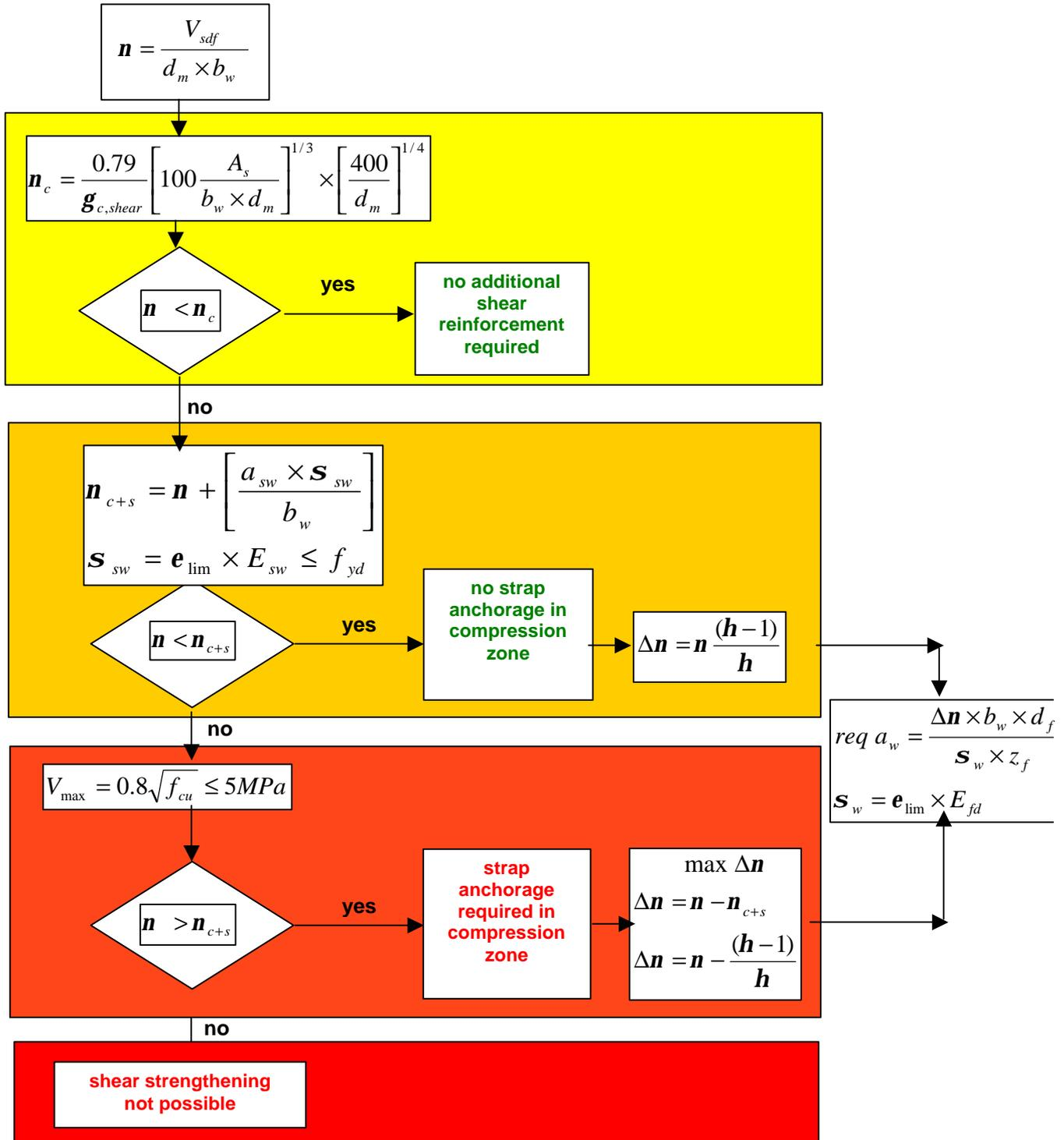
Fig 7.3: Flowchart for check of shear, according to BS 8110 [R7.8]
