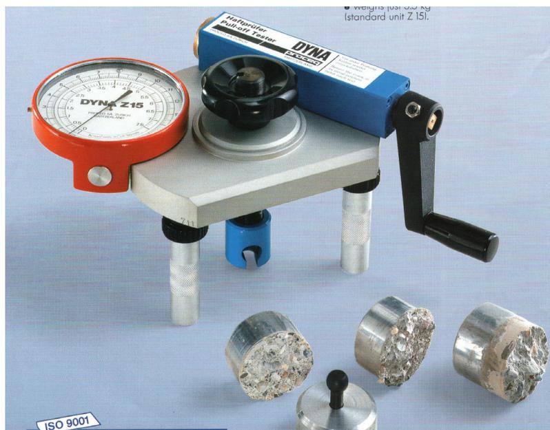
Fig 3.1: Proceq Dyna Pull-off Tester used for determining substrate tensile strength
