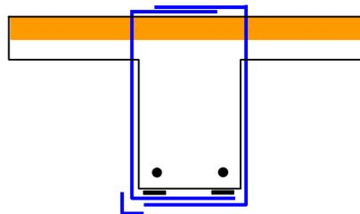
**Fig 7.6: Anchorage in the compression zone required**
