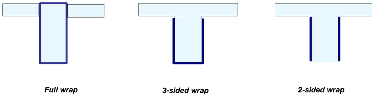
**Fig 7.1: Types of wrapping systems for shear enhancement**
