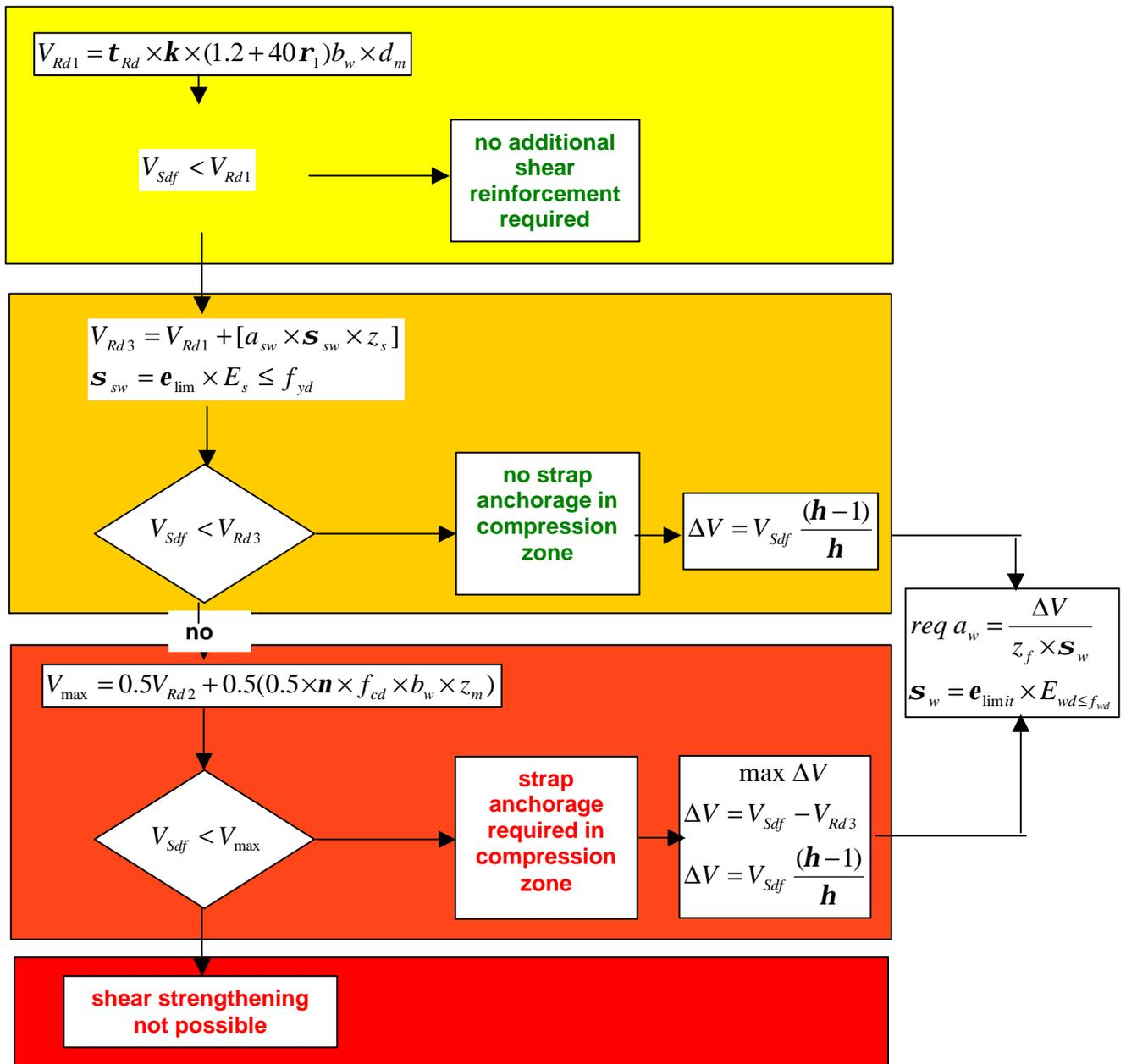
Fig 7.7: Flowchart for check of shear, according to EC2
