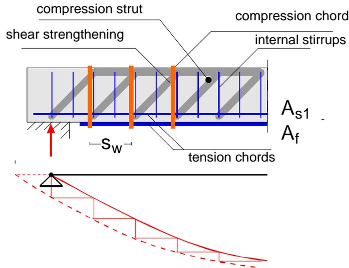
**Fig. 7.5: Connection of the FRP shear strengthening to the internal truss structure [R7.8]**
