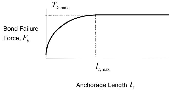
**Fig 6.5 : Characteristic bond failure force vs anchorage length**
