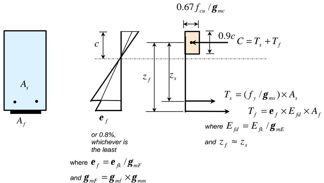
**Figure 6.2: Design Moment less than Balanced Failure Moment using UK Concrete Society TR55 Guidelines and BS 8110**
