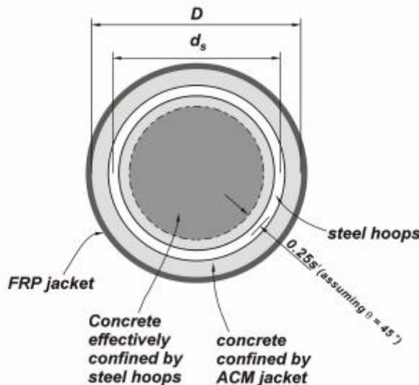
**Figure 8.2 Dual Confinement Effect on a Circular Column with an FRP Jacket and Internal Steel Hoops**
