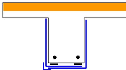
**Fig 7.4: No anchorage in the compression zone**
