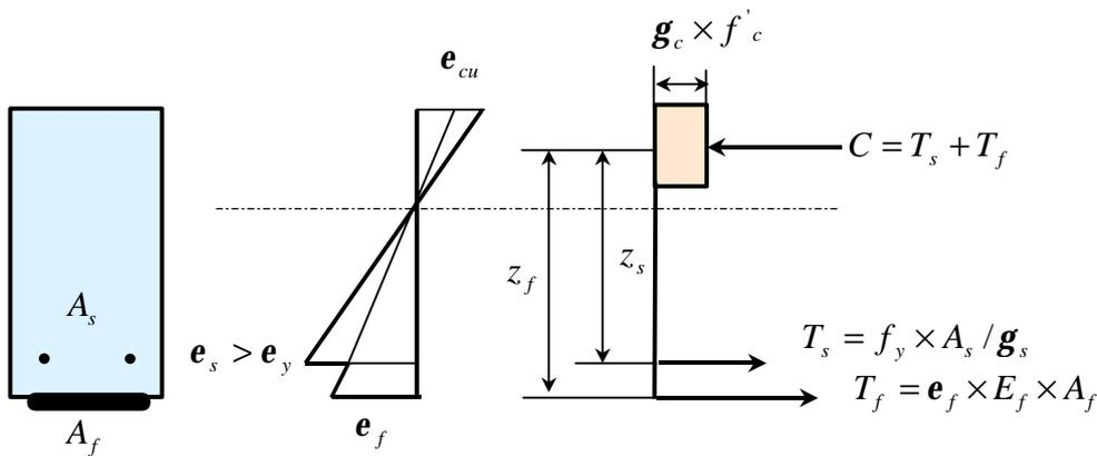
Figure 6.4: Design Moment less than Balanced Failure Moment using German General Guidelines & Eurocode 2
