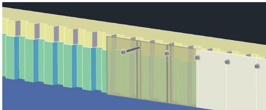
filler capable of bonding to the face of the steel and resisting the compressive stresses imposed by static water head and wave action. It would also need to be stable in a marine environment, resistant to attack from seawater and marine organisms.
