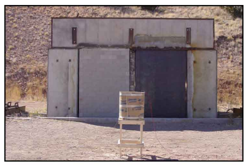
Figure 2: URM wall test specimens ready for blast test
